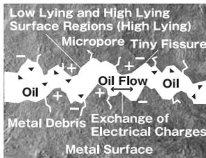
Friction between metals causes electrification, which gives the high lying region (+) charges and the low lying region (-) charges.
